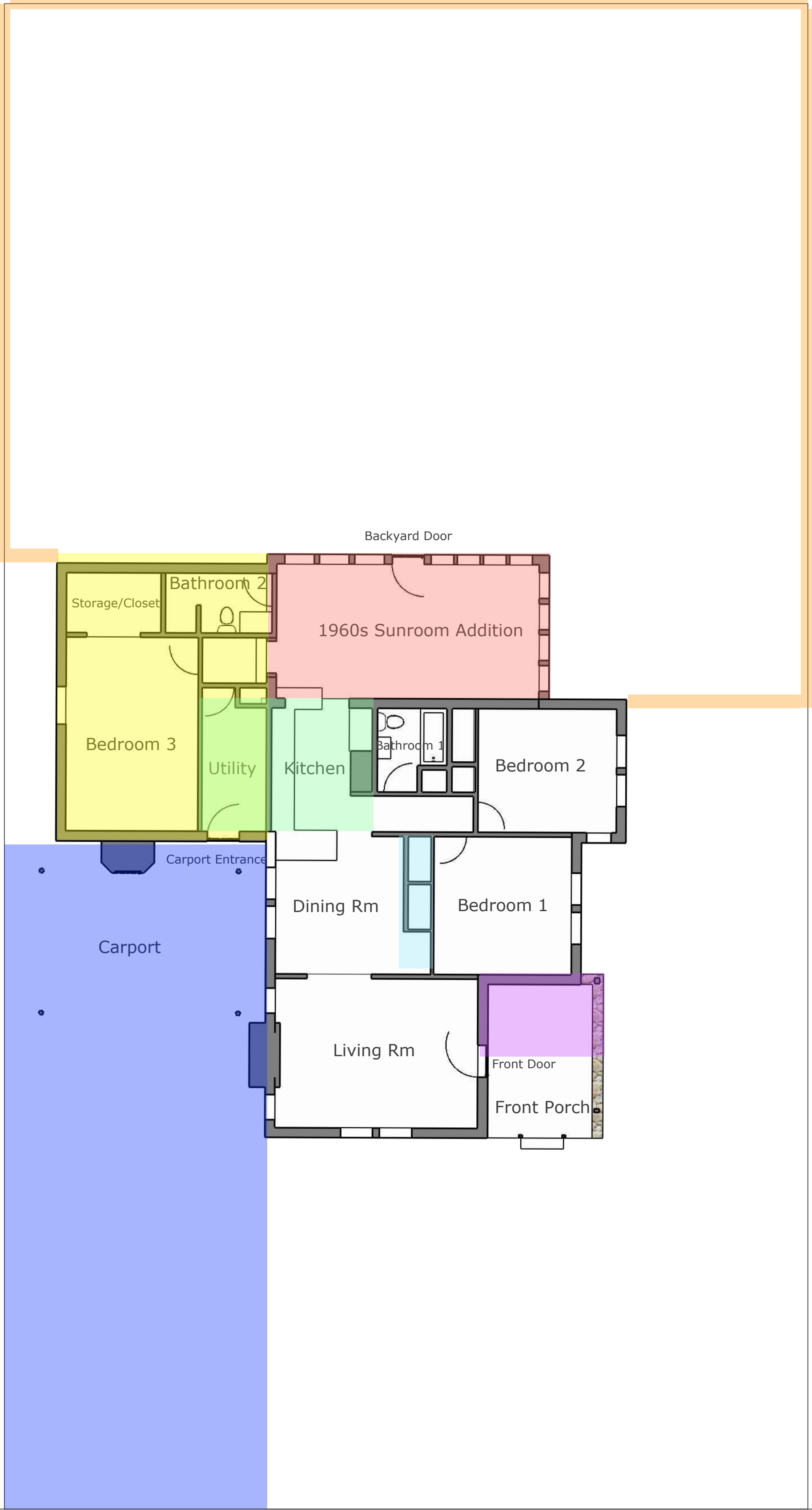
Original House Floor Plan (shown with Property Bounds) SCALE: 1/8" = 1' (1:96)
